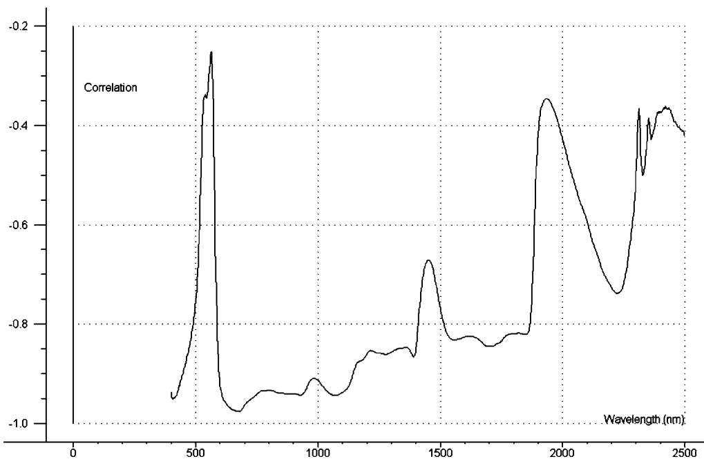
Figure 3. Correlogram between wavelength data and adulteration class for the blue swimmer and Atlantic blue crab meat data set.
